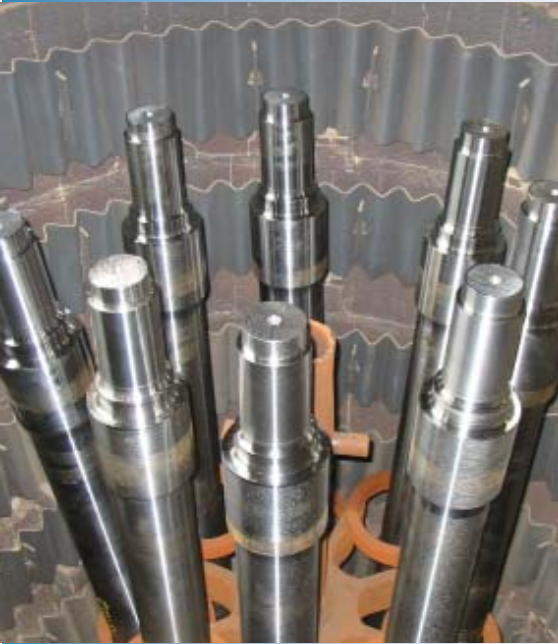
Axles positioned for the subcritical quenching process in an electric furnace
