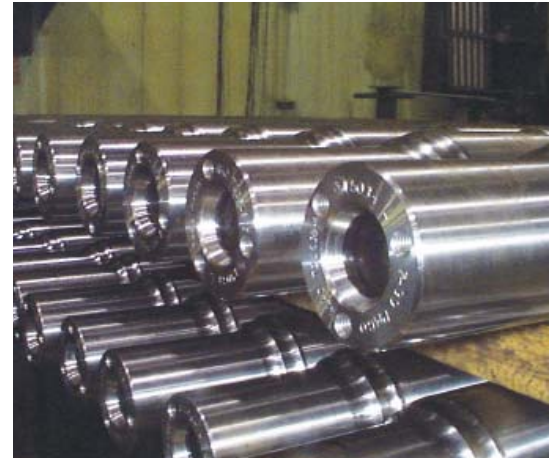
Hollow axles with AAR stamping
