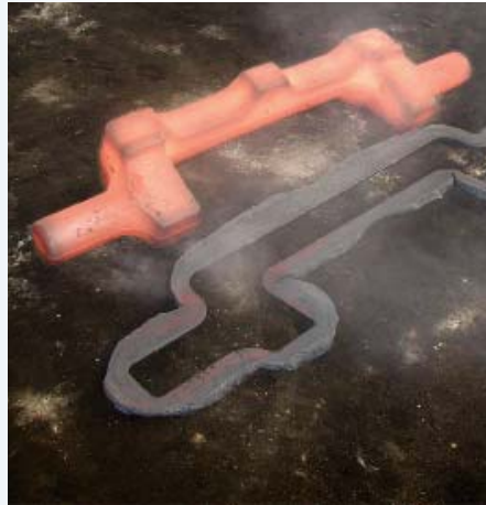
Cast low-floor axle after removal from the die
