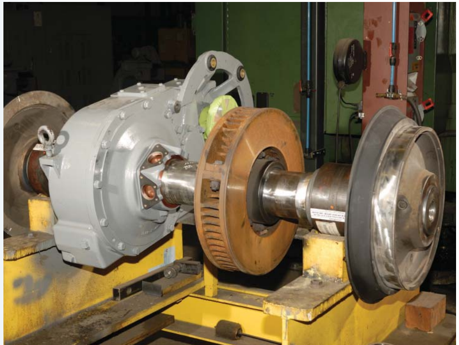
Penn Machine's wheel/axle presses, designed specifically for transit applications, precisely assemble wheel sets.
