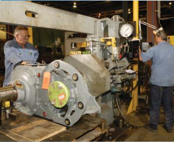
Penn Machine's wheel/axle presses, designed specifically for transit applications, precisely assemble wheel sets.
