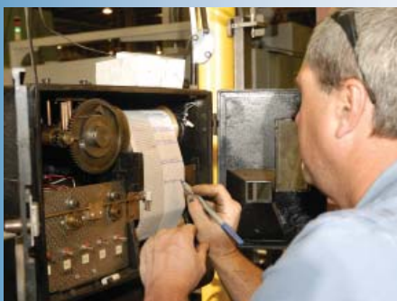
Penn Machine's wheel/axle presses are all equipped with AAR chart recorders.
